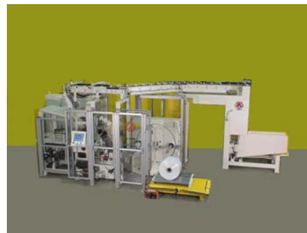
Shown incorporated with Elsner Model AFR Series Rewinder for Kitchen Rolled Products
